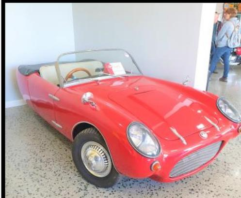
**A Berkeley T60 three wheel sports car from England; front wheel drive powered by a 328 cc air cooled twin cylinder engine through a 4 speed gearbox.**
